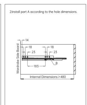
3.Secure A to the side board with B, ensuring that A on both sides are at the same horizontal level.
